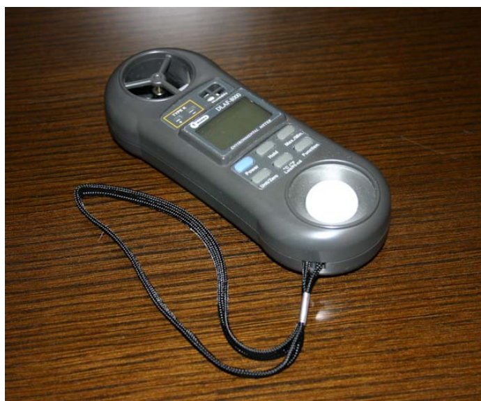
Figure 11. Environmental meter used to collect humidity, temperature, and lighting values.
